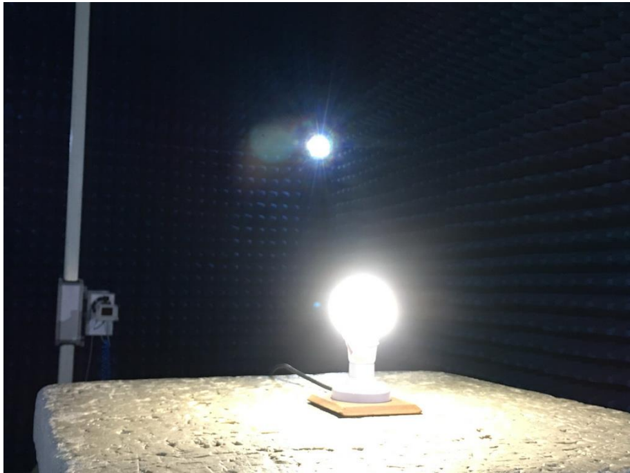
Photograph 7: Set-up for Radiated Spurious Emission, 18GHz - 26.5GHz
