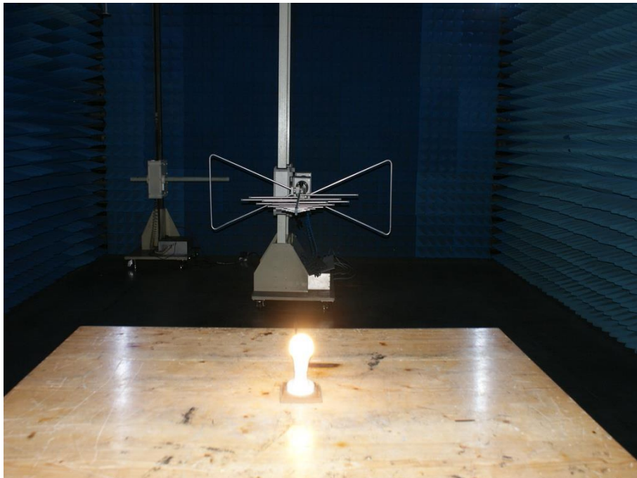
Photograph 2: Set-up for Radiated Emission, below 1GHz
