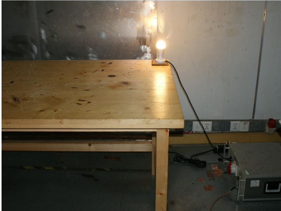
Photograph 1: Set-up for Conducted Emission on AC Mains
