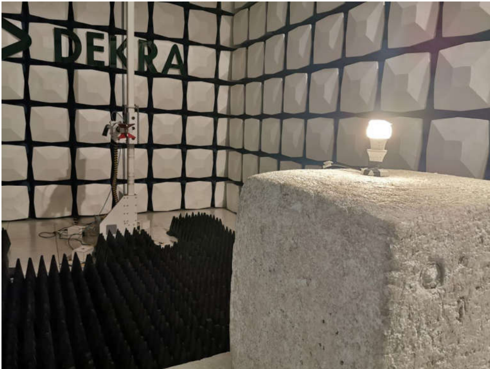
Description: Radiated Emission Test Setup for 1~18GHz
