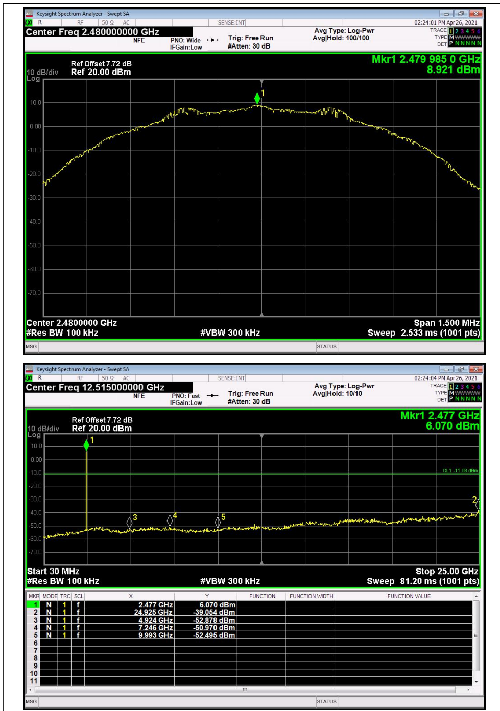
(LE 1M PHY _ Conducted Spurious Emissions _ Channel = 39, 30MHz to 25GHz)
