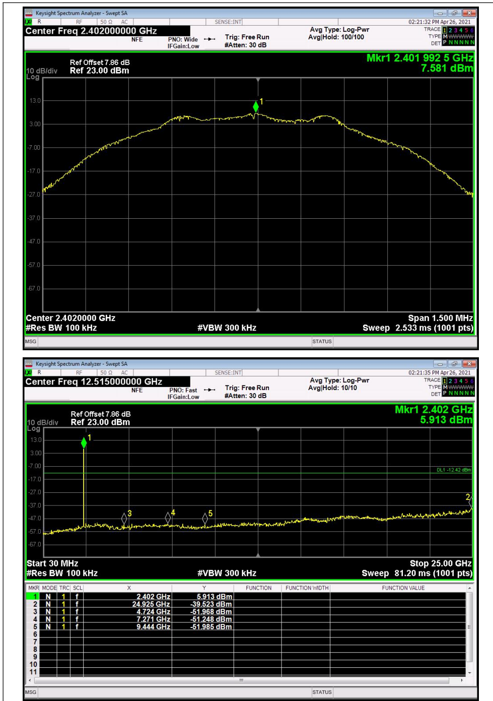
(LE 1M PHY _ Conducted Spurious Emissions _ Channel = 0, 30MHz to 25GHz)
