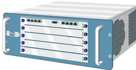
Figure 2 The NCU is the main controller of the RFS.
