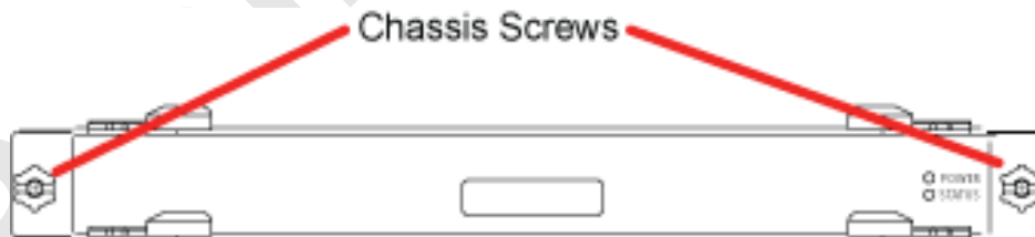
Figure 9.7 Replacing the BPC
