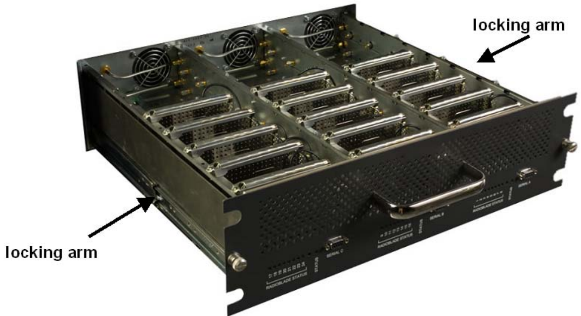
Figure 5.1 Location of DRBS Side Rail Locking Arms
