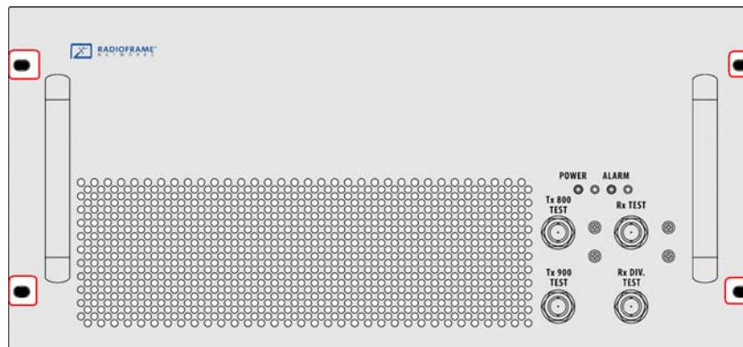
Figure 6.2 RF Shelf Mounting Screw Locations
