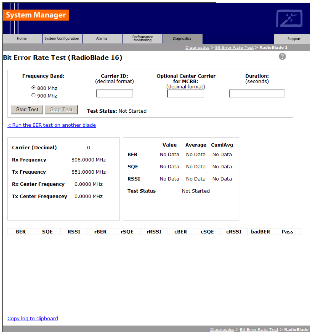
Figure F-6 Bit Error Rate Start Test Page
