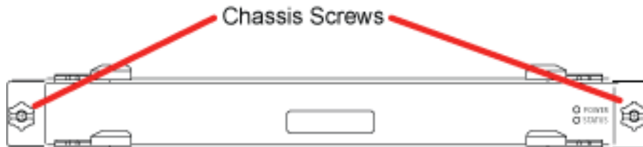
Figure 6.7 Replacing the BPC
