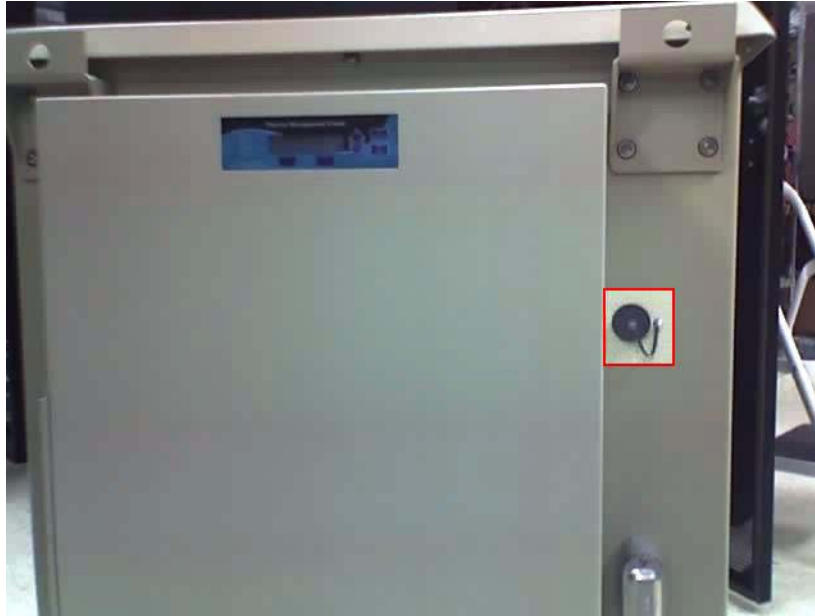
Figure 1.5 Remote RJ-45 System Access from outside the Cabinet
