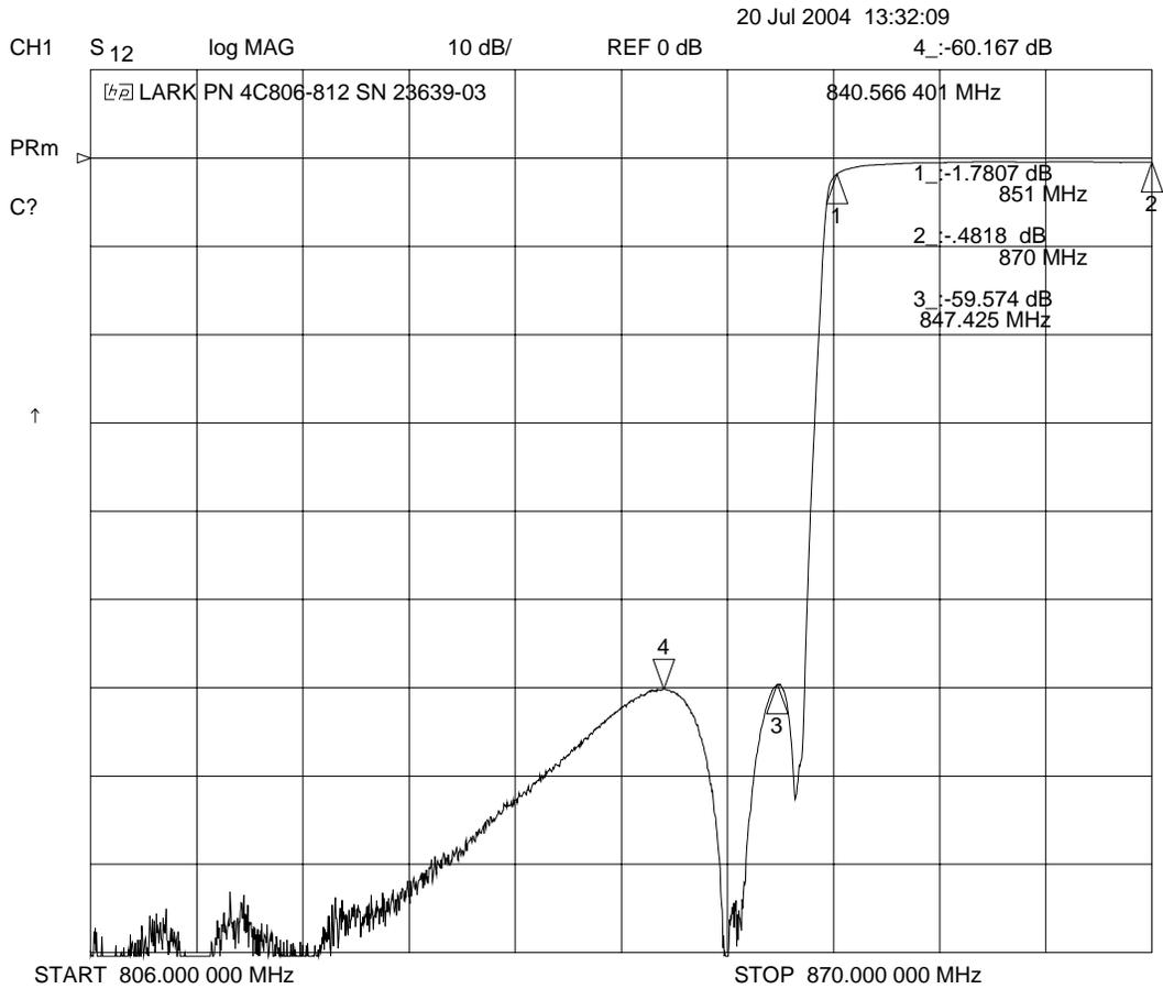
**Figure 43** Transmit filter frequency response
