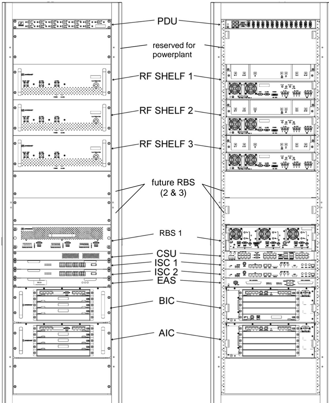
Figure 26 MC-Series System rack locations for non-RFN hardware
