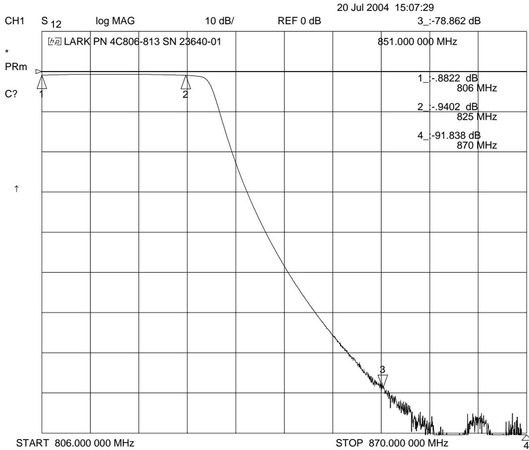
**Figure 44** Receive filter frequency response
