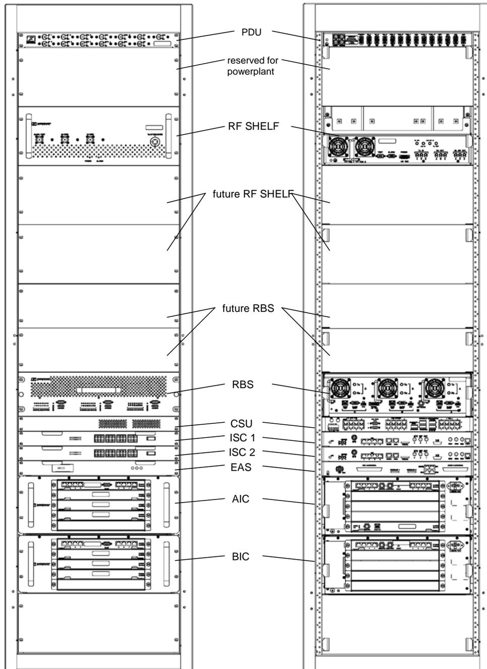
Figure 42 MC-Series System Omni Configuration
