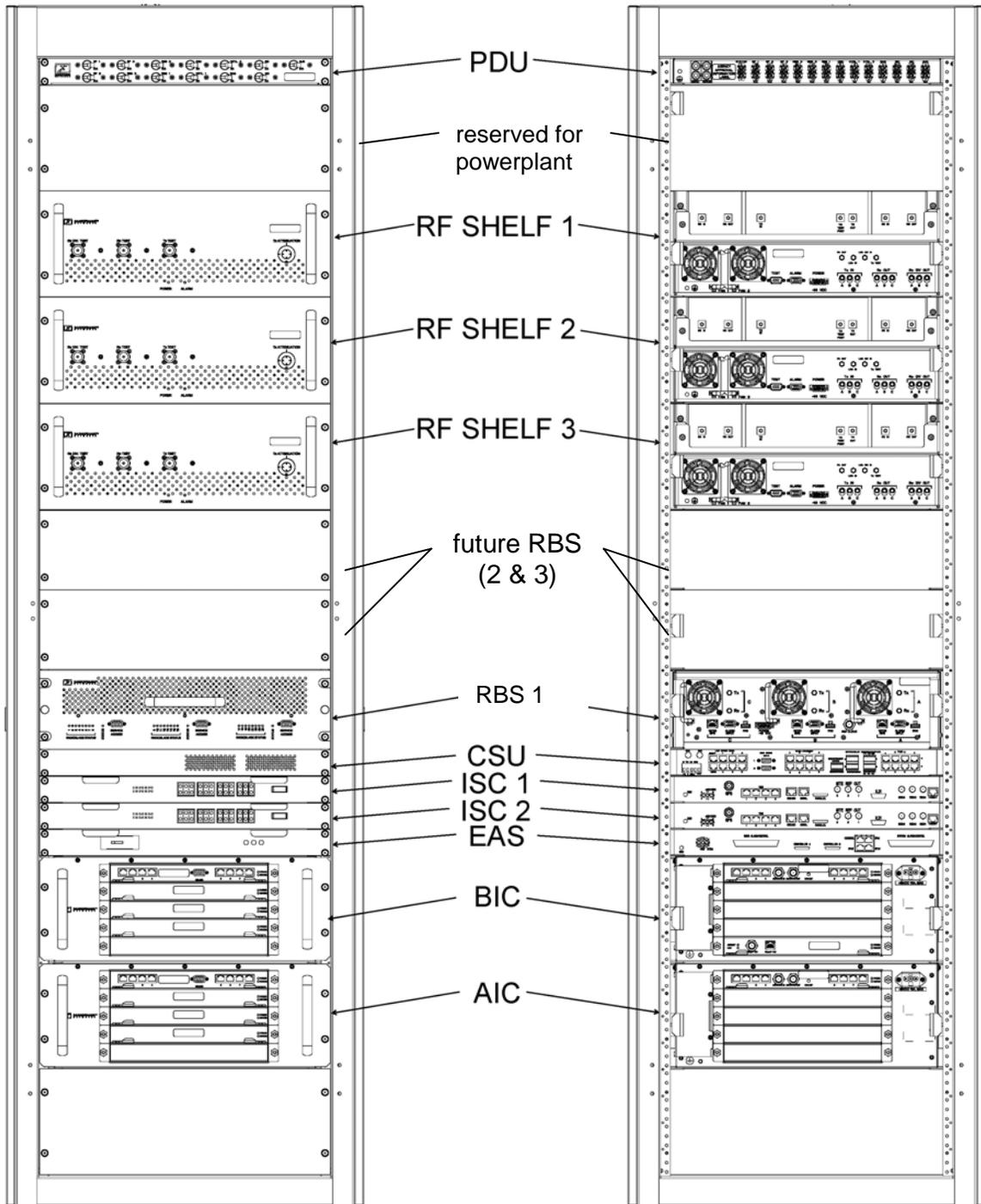
Figure 2 MC-Series System 3-sector configuration
