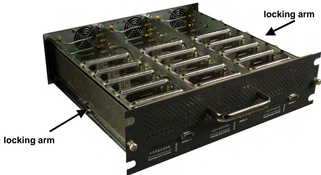
Figure 71 RF Shelf Showing Side-Rail Locking Arm Locations
