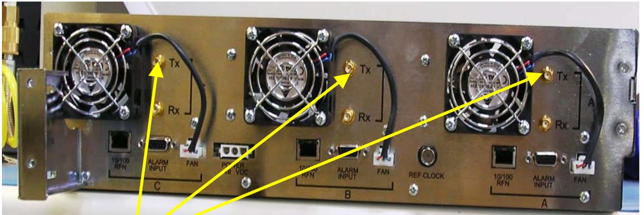
Transmit Signals out from Radios
