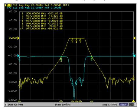
Figure 77 900 MHz Transmit Filter Frequency Response
