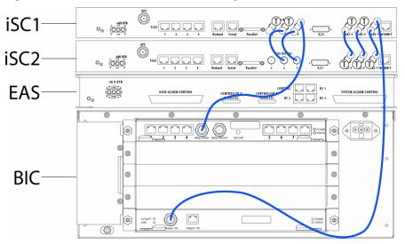
Figure 27 Connections between the Primary iSC and BIC
