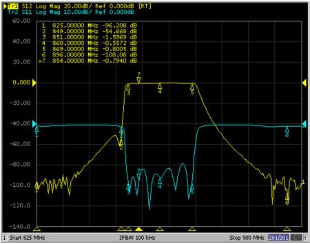
The 900MHz Tx filter response is shown in Figure 77.
