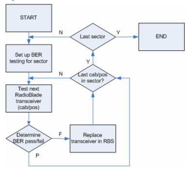
Figure 80 BER Test Flow
