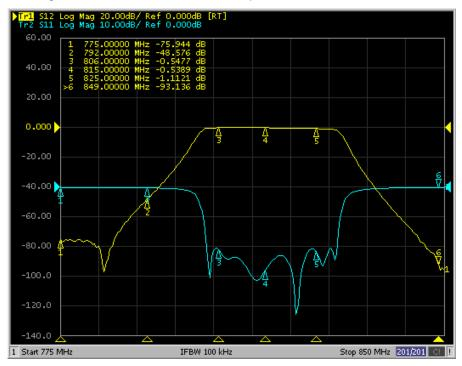
Figure 79 900 MHz Band Rx Filter Response
