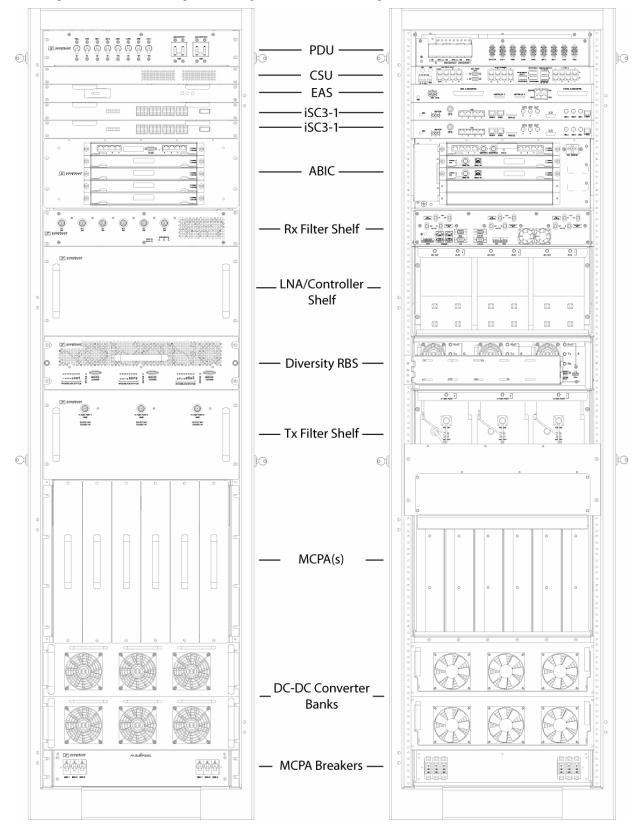
Figure 2 MC-Series High Power System 3-Sector Configuration
