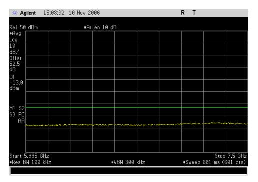
3 Channel Intermods, 7.495 GHz-9.5 GHz **Result:** Pass **Value:** <-25 dBm **Limit:** ≤-13 dBm
