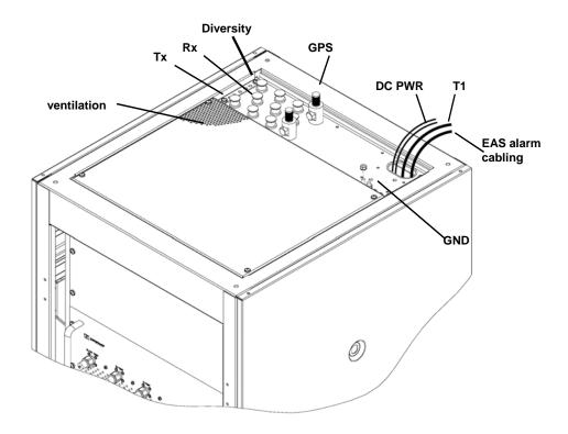
Figure 27 Top of the rack (TOR) cabling and equipment
