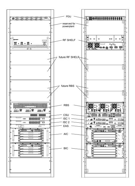
Figure 42 MC-Series System Omni Configuration
