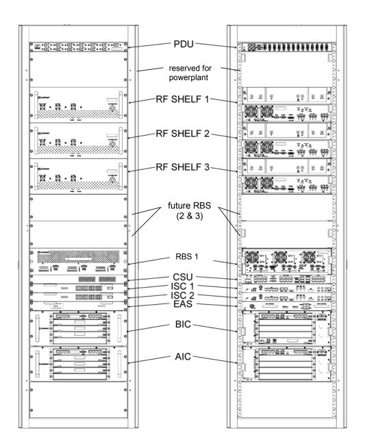
Figure 2 MC-Series System 3-sector configuration
