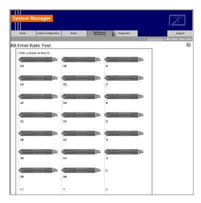
4 For Carrier ID, enter the carrier ID (in decimal format) to which the R2660 is set, and then select the Start Test button.
