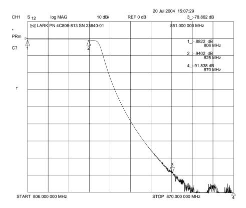
Figure 44 Receive filter frequency response
