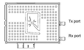
Figure 19 iDEN 2-port RadioBlade transceiver
