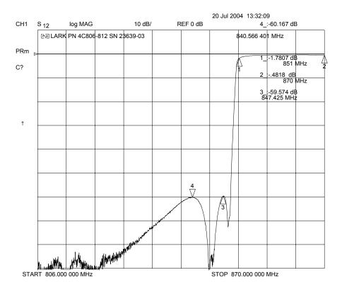
Figure 43 Transmit filter frequency response
