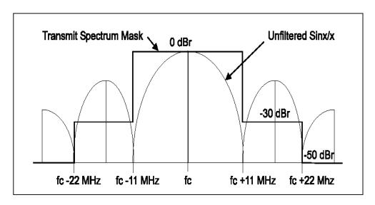
The transmitted spectral products shall be less than -30 dBr (dB relative to the SINx/x peak) for
