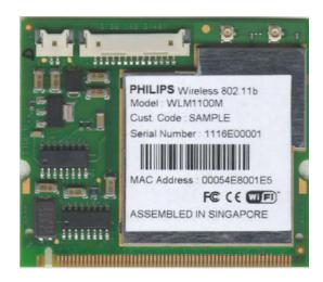
PH10766 - 802.11b Mini PCI Card WLAN
