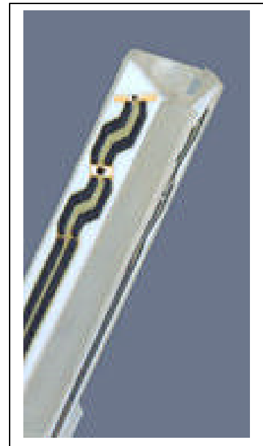
Figure. Inside view of ET3DV6 E-field Probe
