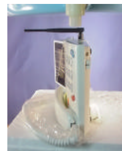
Body SAR Test Setup 3.0cm Separation Distance
