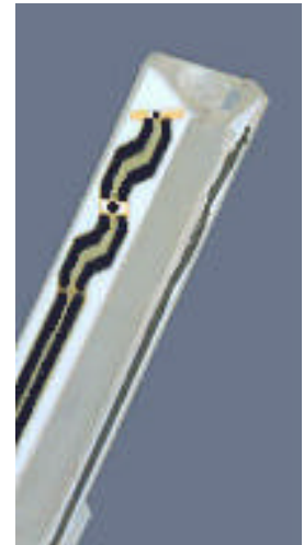
ET3DV6 E-Field Probe
