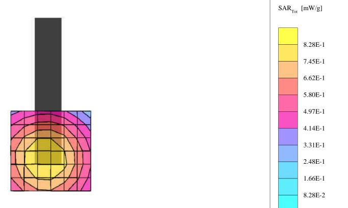
$\begin{array}{c} GPRS \ 2 \ Slot \ Uplink \ \text{-} \ DELL \\ 0 \ \text{Degrees to Phantom with Antenna Up Bottom Channel (512)} \\ SAM \ Phantom; \ Flat \\ Probe: \ ET3DV6 \ \text{-} \ SN1529; \ ConvF(4.70,4.70,4.70); \\ Crest \ factor: \ 4.0; \ Body \ 1900MHz \ FCC: \ \sigma = 1.58 \ mho/m \ \epsilon_r = 52.8 \ \rho = 1.00 \ g/cm^3 \\ Lab \ Temperature \ 22.0 \ deg \ C, \ Fluid \ Temperature \ 18.9 \ deg \ C \\ SAR \ Drift \ 9.78\% \\ 01/21/03 \end{array}$
