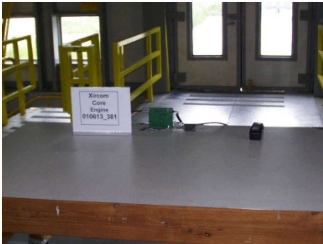
Figure E14.2. Radiated Emissions set-up at Criterion Technologies.
