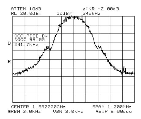
Figure E12.1. Occupied bandwidth measurement result, channel 661(1880.0MHz).
