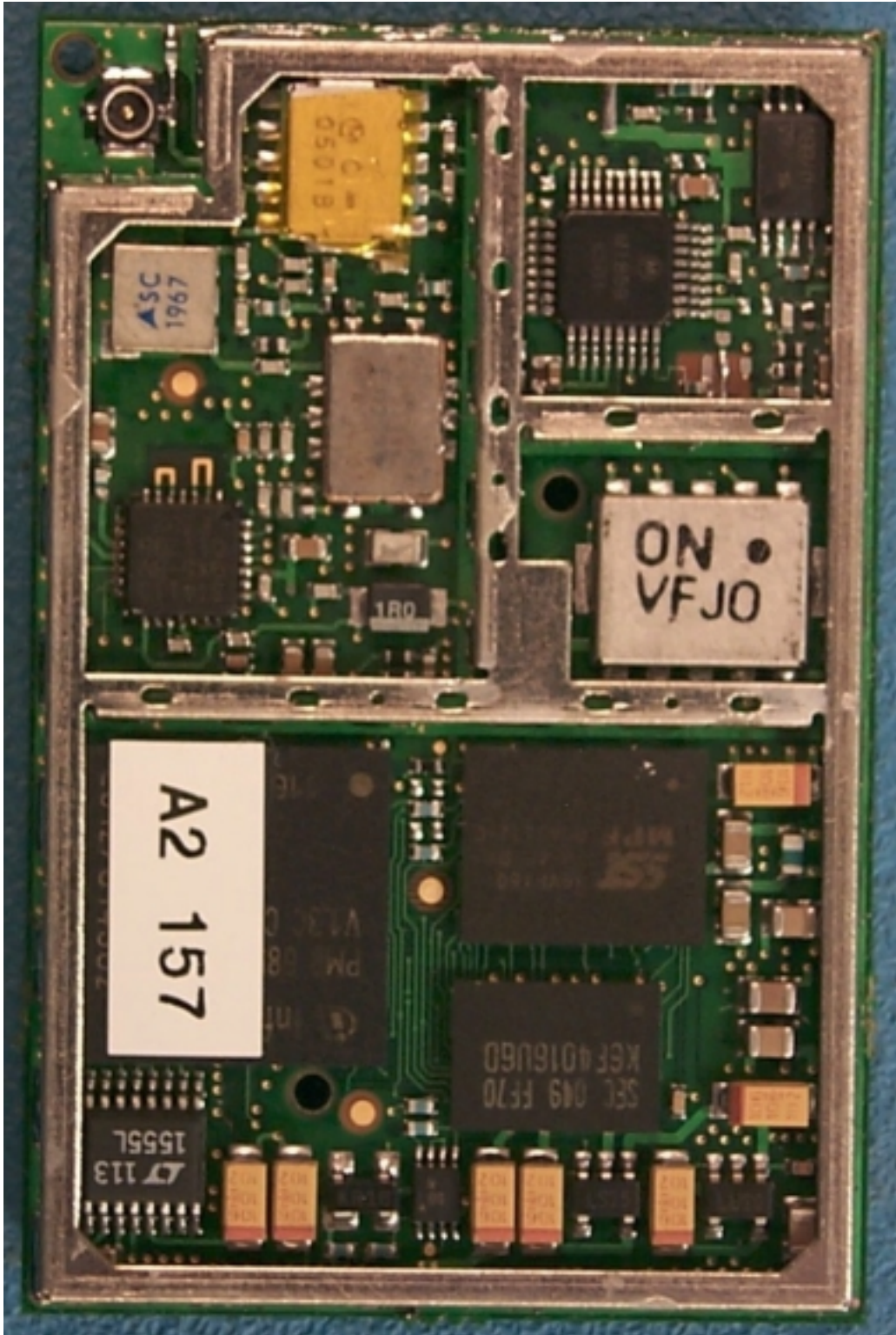
Photo 1. Top of Core Engine PCB (shields removed).
