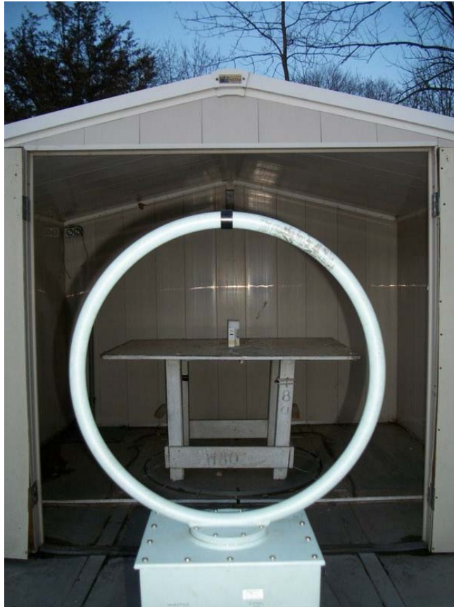
Figure 3.1 Radiated Test Setup
