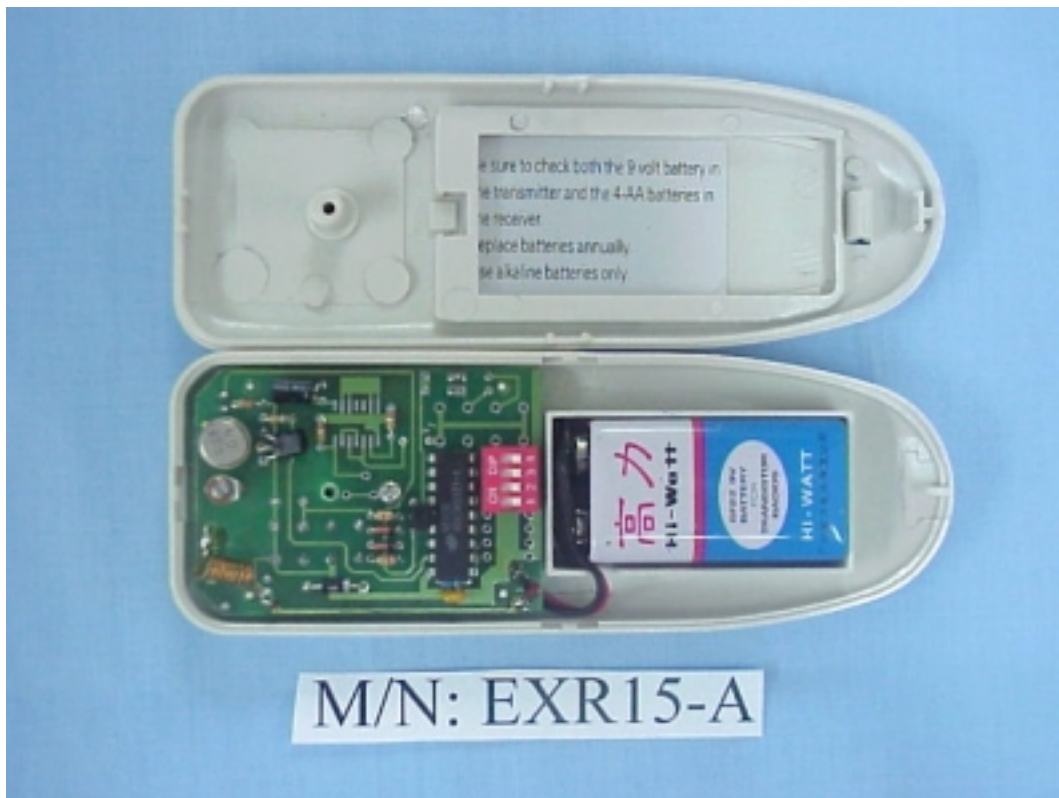
FIGURE 1 RADIO REMOTE CONTROLLER (M/N: ERX15-A) COVER REMOVED
