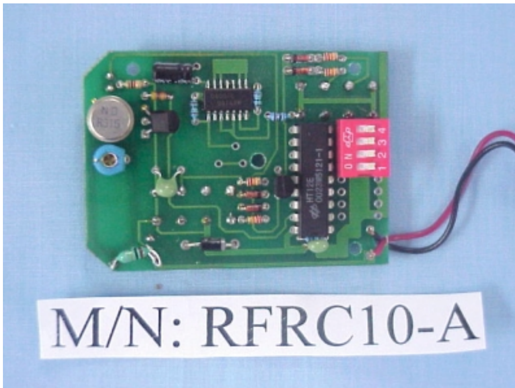
FIGURE 6 RADIO REMOTE CONTROLLER (M/N: RFRC10-A) SOLDERED SIDE
