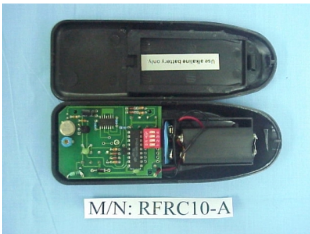
FIGURE 4 RADIO REMOTE CONTROLLER (M/N: RFRC10-A) COVER REMOVED
