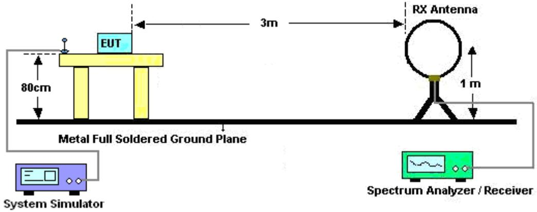
For radiated emissions from 30MHz to 1GHz
