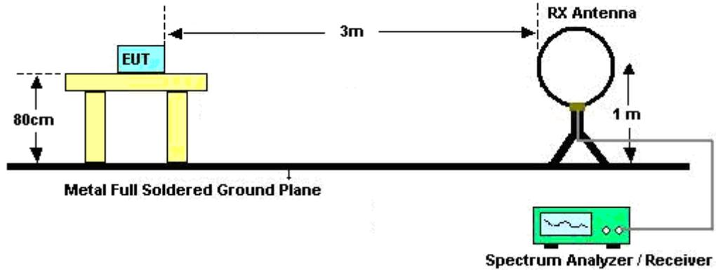
For radiated emissions from 30MHz to 1GHz
