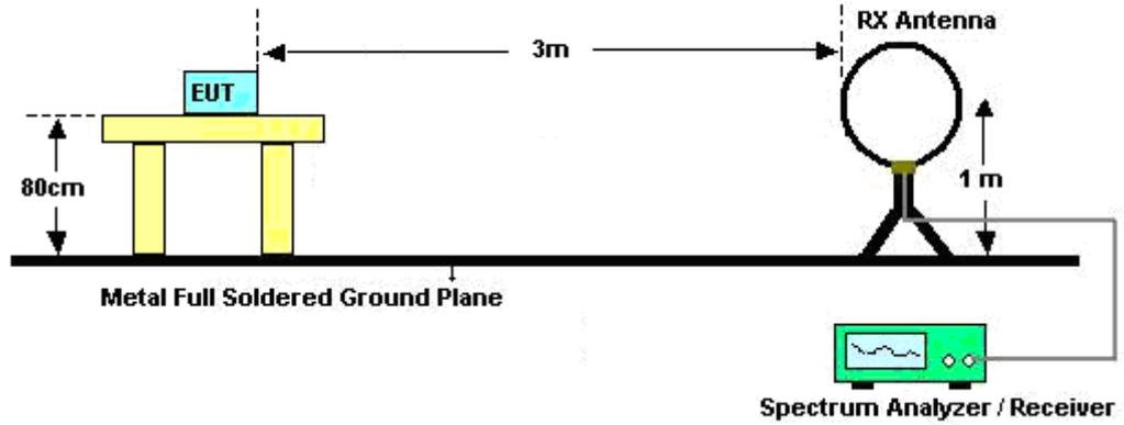
For radiated emissions from 30MHz to 1GHz
