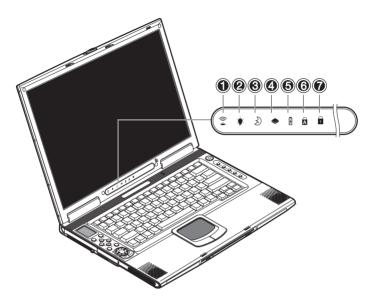
The Power and Standby indicators are visible even when you close the display cover so you can see the status of the computer while the cover is closed.
