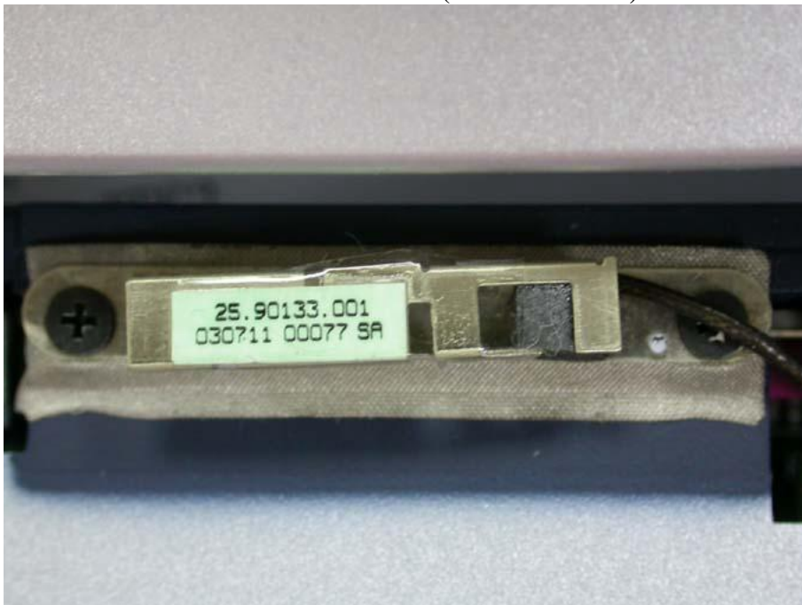
Photo of Main Antenna (RF TX Antenna)
