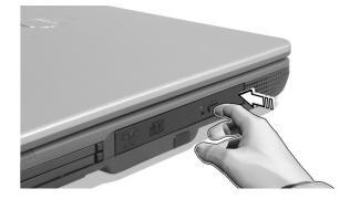
When the power is off, you can eject the drive tray using the emergency eject hole. See page 65.
