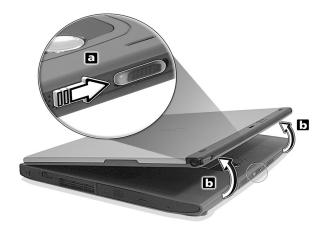
2 Open the display screen to an angle of about 90 degrees. When viewed from the side, the display should be perpendicular to the computer base.
