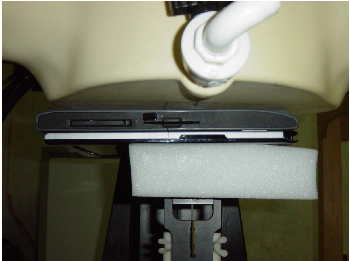
802.11a (OFDM): Duty Cycle = 100%, Crest Factor: 1. Depth of liquid: 15.0 cm
