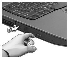
When the power is off, you can eject the drive tray using the emergency eject hole. See page 54.
