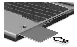
To remove the Smart Card press the Smart Card eject button (a) and remove the Smart Card (b) as shown in the illustration below.
