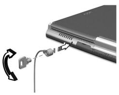
Wrap a computer security lock cable around an immovable object such as a table or locked drawer handle. Insert the lock into the notch and turn the key to secure the lock. Some keyless models are also available.
