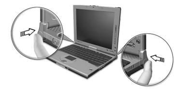
**3** Rotate the display screen 180 degrees clockwise as shown in the illustration. Make sure that the display screen is aligned with the screen supports that will hold it in place.
