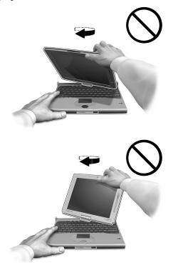
2 Press and release the screen support holding the display screen on both sides.
