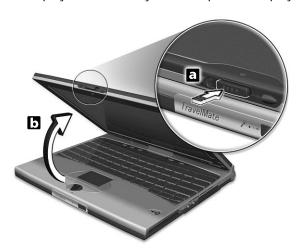
4 Slide the power switch towards the rear of the computer (a) then release it (b) to turn on the power. The POST (power-on self-test) routine executes and Windows begins loading.
