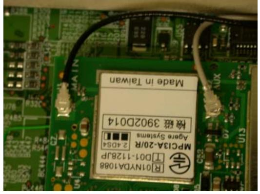
(The white wire (AUX) is connected to the bottom antenna)
