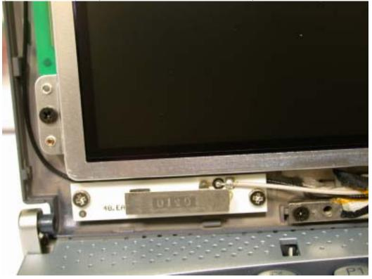
(The black wire (MAIN) is connected to the top antenna.)
