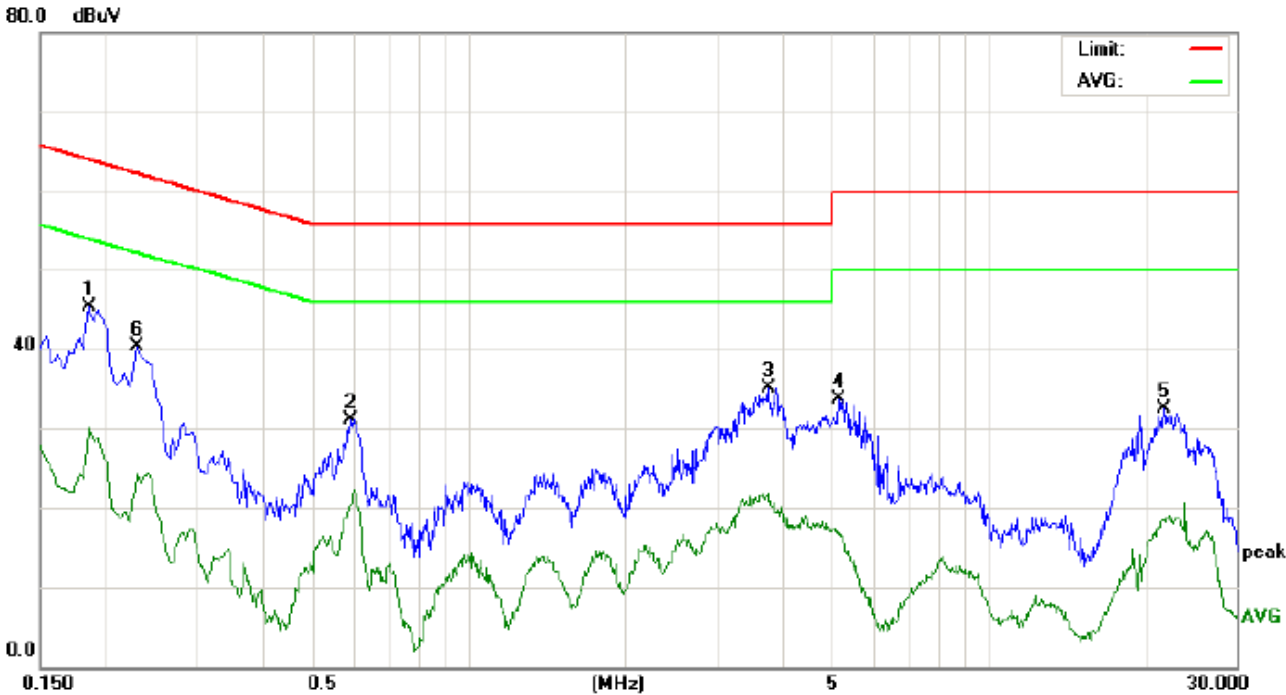
Line Conducted Emission Test Line 1-L
