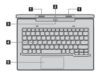
**Tablet-docking latch** Connects the tablet to the dock and keeps the tablet secured in place.
