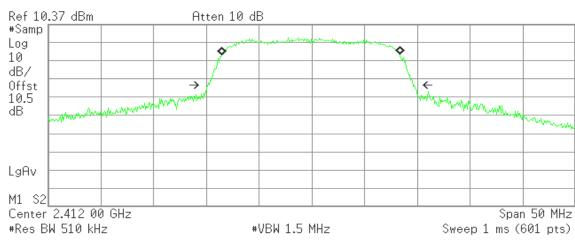
Occupied Bandwidth 16.7572 MHz Occ BW % Pwr 99.00 % x dB -26.00 dB
