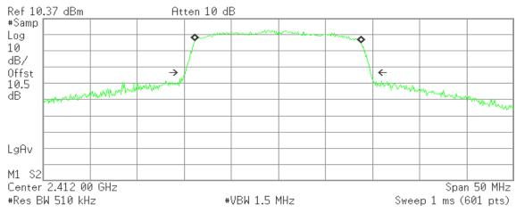
Occupied Bandwidth 17.5928 MHz Occ BW % Pwr 99.00 % x dB -26.00 dB
