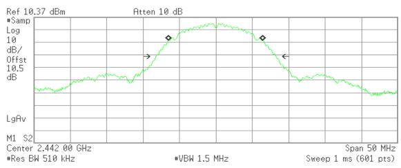
Occupied Bandwidth 12.8833 MHz Occ BW % Pwr 99.00 % x dB -26.00 dB
