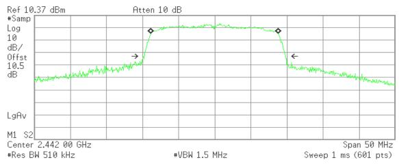
Occupied Bandwidth 17.5757 MHz Occ BW % Pwr 99.00 % x dB -26.00 dB
