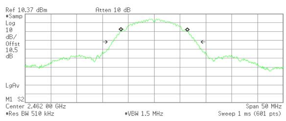
Occupied Bandwidth 12.7920 MHz Occ BW % Pwr 99.00 % x dB -26.00 dB
