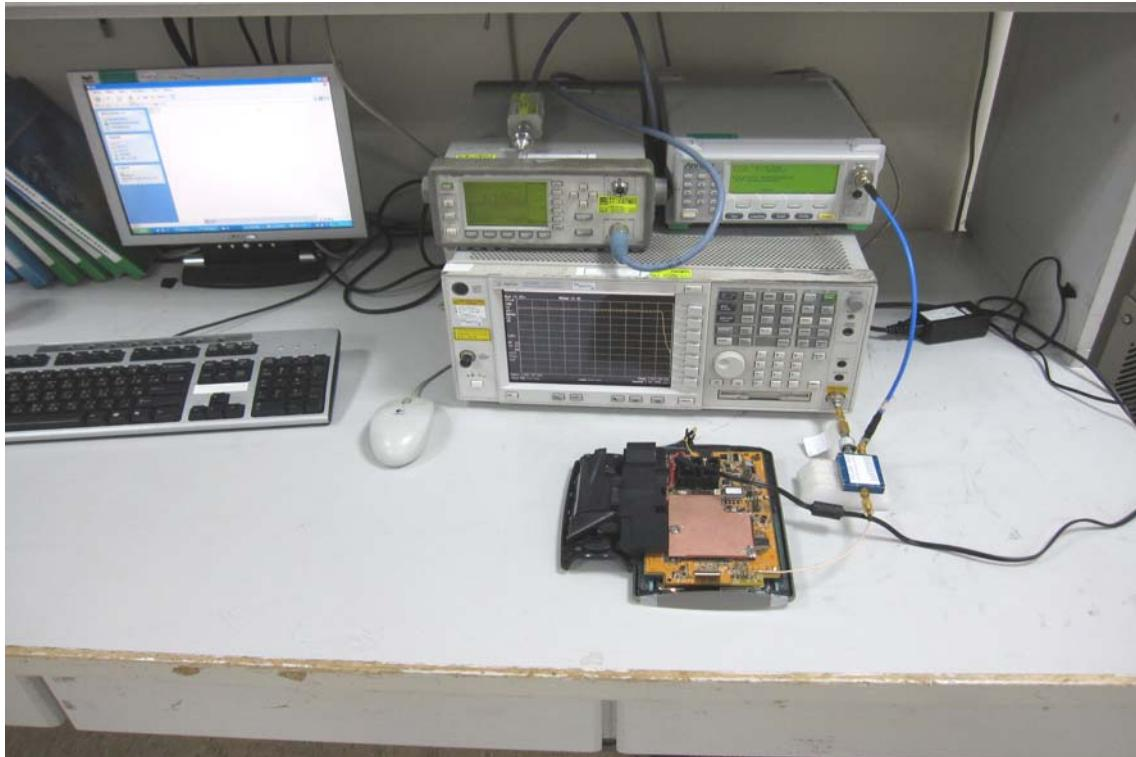
**RADIATED EMISSION SETUP PHOTOS****Below 1 GHz**
