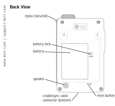
**BATTERY LOCK** — Use this switch to release and remove the main battery. See "Installing and Removing the Battery" on page 25.
