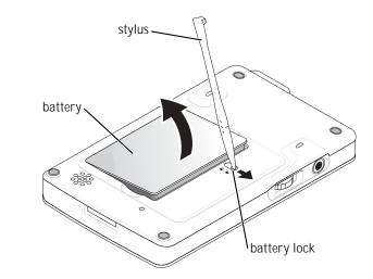
**NOTE:** Your service tag is located underneath the battery. You need your service tag if you access Dell Support at **support.dell.com** or if you call Dell for customer service or technical support.
