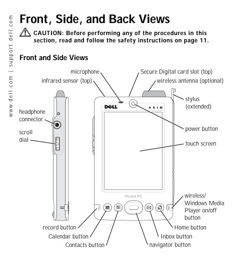
**INFRARED SENSOR** — The infrared sensor lets you transfer files from your device to another infrared-compatible device without using cable connections.
