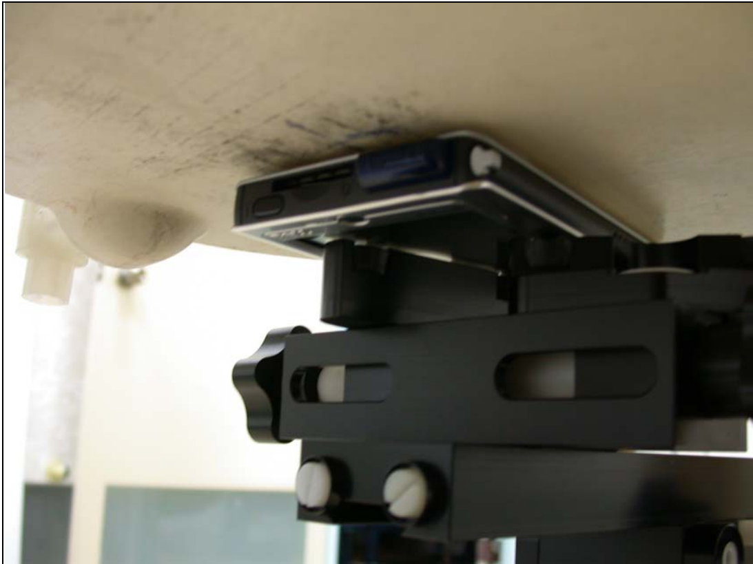
The bottom side of the EUT to the flat phantom distance 0mm
