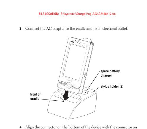
the cradle, and, keeping the front of the device flush with the front of the cradle, lower the device onto the cradle.
