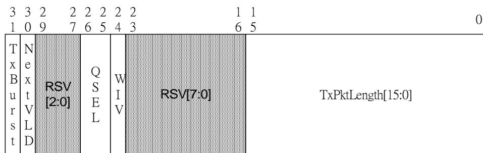
TXINF is prepared by host driver and used for passing information to DMA. Its size is 1 DW and put at the head of each Tx frame. Following is the detail description of each field of TXINF:
