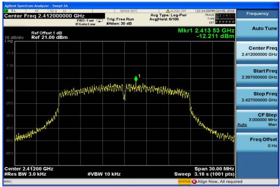
**Power Spectral Density Test Plot (CH-Mid)**
