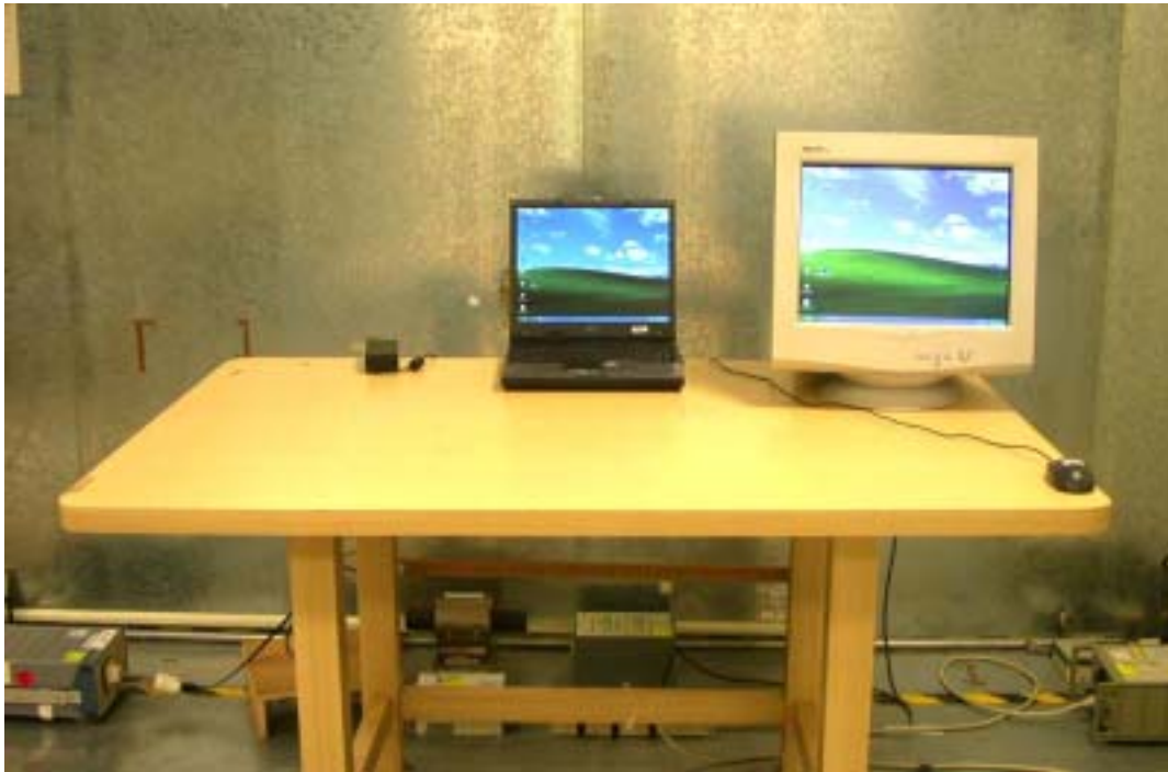
The Front View of Highest Conducted Set-up For EUT
