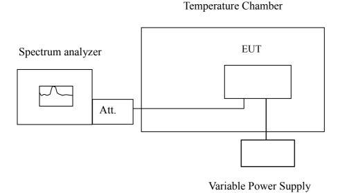
Remark: Measurement setup for testing on Antenna connector
