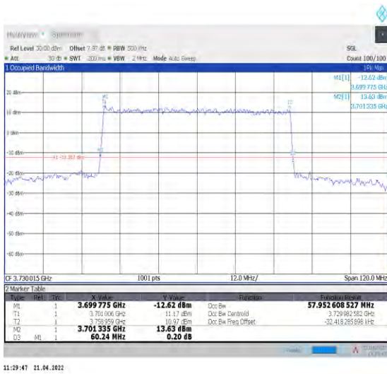
1-N78-3700-3800--30-60-L-3-DFT-16QAM-Outer_Full I-162@0-Ant1-57.953-60.240-≤60-PASS
