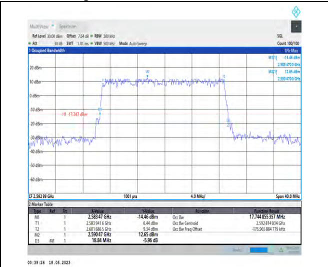
1-N41-PC1-30-20-M-5-DFT-256QAM-Outer_Full-50@ 0-Ant1-17.745-18.840-≤20-PASS
