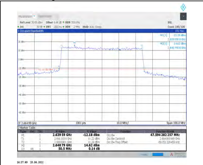
1-N41--30-50-H-7-CP-16QAM-Outer_Full-133@0-An t1-47.594-50.500-≤50-PASS
