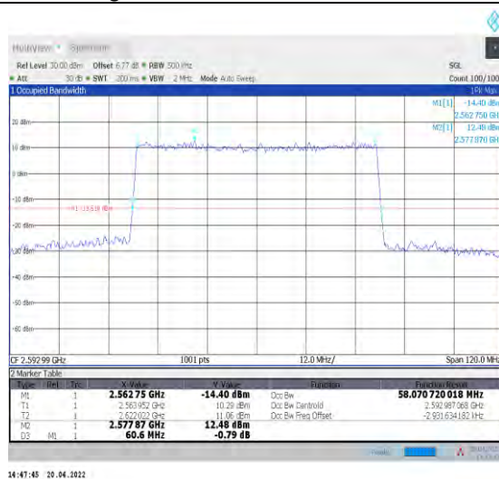
1-N41--30-60-M-5-DFT-256QAM-Outer_Full-162@0-A Ant1-58.071-60.600-≤60-PASS
