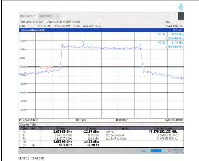
1-N41--30-50-H-8-CP-64QAM-Outer_Full-133@0-An t1-47.579-50.300-≤50-PASS
