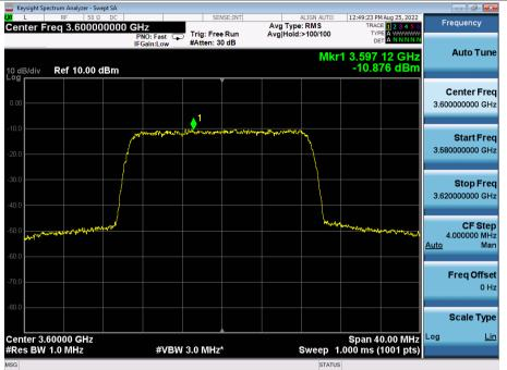
EIRP PSD=-10.876-6.1+15=-1.976dBm/MHz, attenuation of Cable and Splitter is 15dB, Antenna gain is -6.1dBi.
