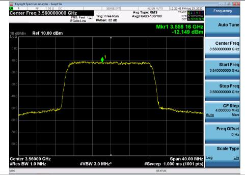
EIRP PSD=-12.149-6.1+15=-3.249dBm/MHz, attenuation of Cable and Splitter is 15dB, Antenna gain is -6.1dBi.
