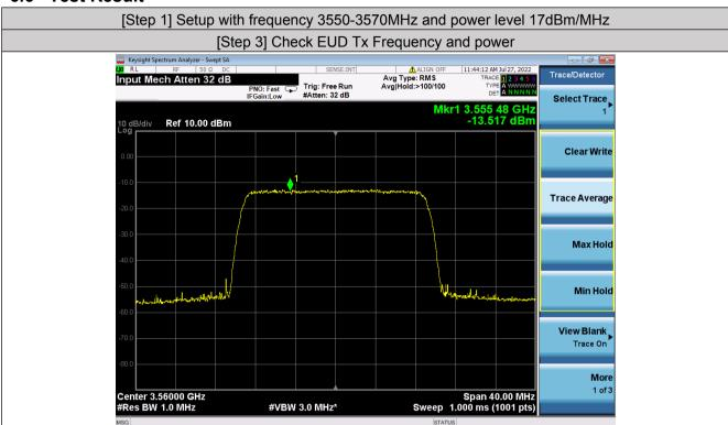
EIRP PSD=-13.517-6.1+15=-4.617dBm/MHz, attenuation of Cable and Splitter is 15dB, Antenna gain is - 6.1dBi.
