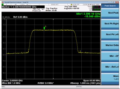
EIRP PSD=-18.049-6.1+15=-9.149dBm/MHz, attenuation of Cable and Splitter is 15dB, Antenna gain is - 6.1dBi.
