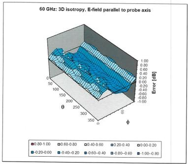
Probe isotropy for E<sub>tot</sub>: probe rotated  $\phi$  = 0° to 360°, tilted from field propagation direction  $\overline{k}$  Parallel to the field propagation ( $\psi$  =0° - 90°) at 30 GHz: deviation within ± 0.36 dB Parallel to the field propagation ( $\psi$  =0° - 90°) at 60 GHz: deviation within ± 0.37 dB
