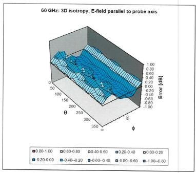
Probe isotropy for E<sub>tot</sub>: probe rotated  $\phi$  = 0° to 360°, tilted from field propagation direction  $\overline{k}$  Parallel to the field propagation ( $\psi$  =0° - 90°) at 30 GHz: deviation within ± 0.36 dB Parallel to the field propagation ( $\psi$  =0° - 90°) at 60 GHz: deviation within ± 0.37 dB
