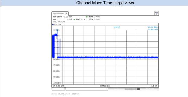
Marker M1 shows the end of the radar signal. Channel move time < 10s. Test PASS
